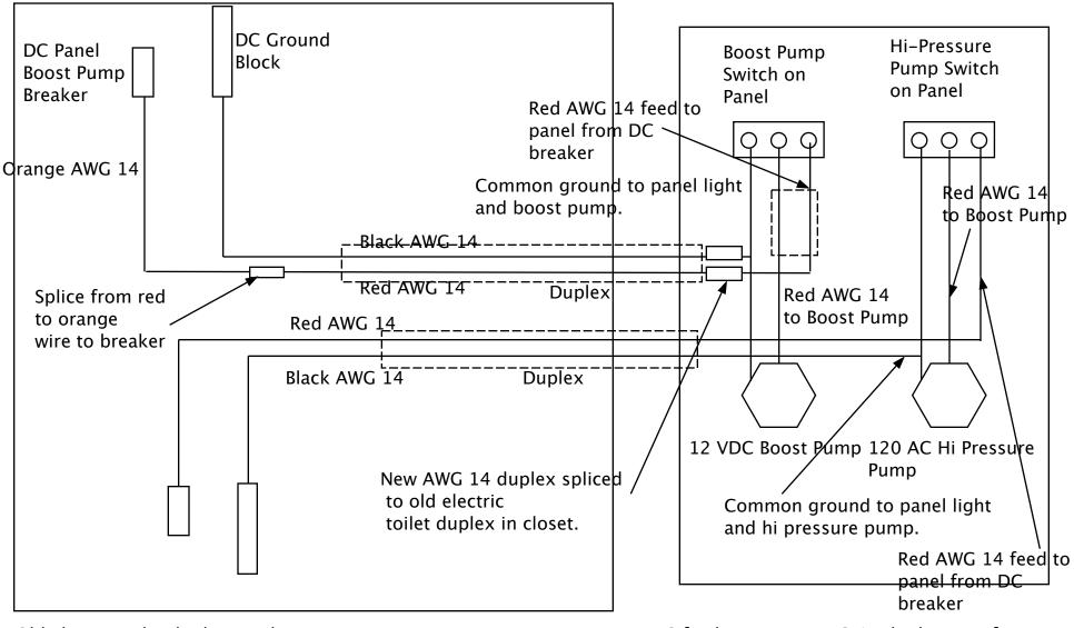
Old electric toilet duplex used. Off-white duplex through outside hole from water maker locker into nav station back. AC feed uses new AWG 14 duplex wire from AC breaker to panel. Uses new inside hole to penetrate to nav station.
